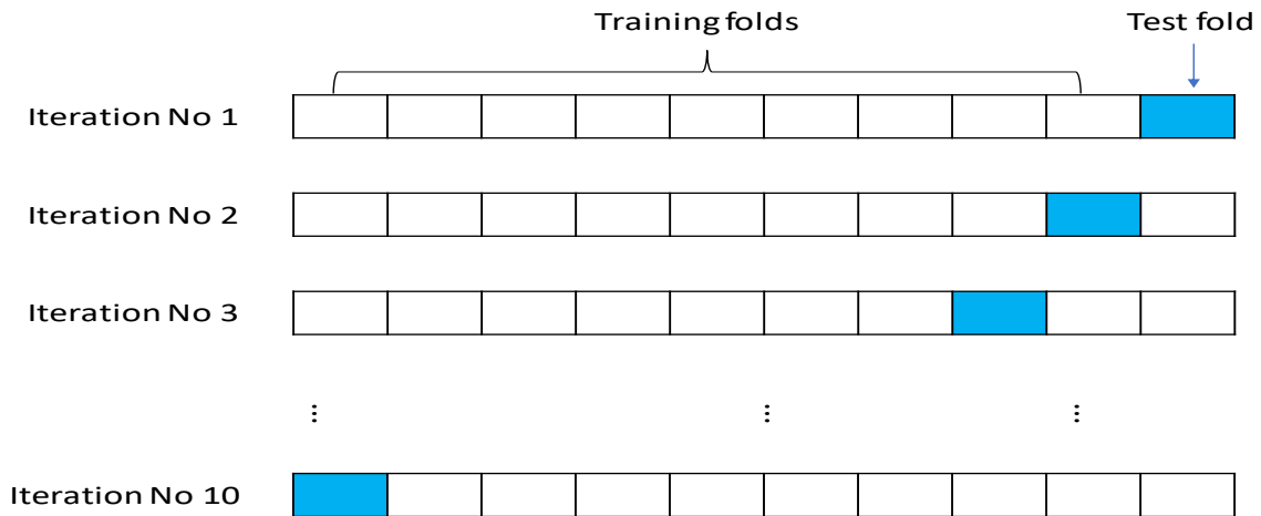
Figure 3.6 Illustration of k-fold (10-fold) cross-validation.
