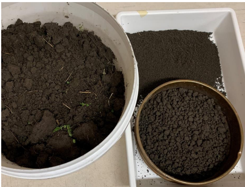
Figure 3.2 Collected field soil samples were sieved through a 2 mm mesh.
