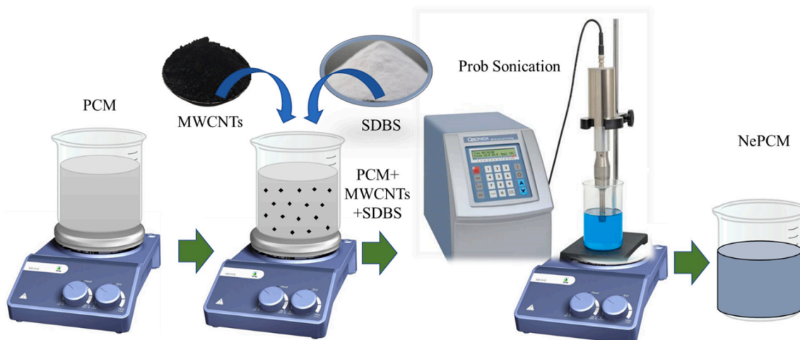
Fig. 1. Fabrication method of nano-enhanced PCM with and without surfactant.
