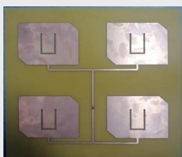
Figure-3. Fabricated microstrip antenna array
