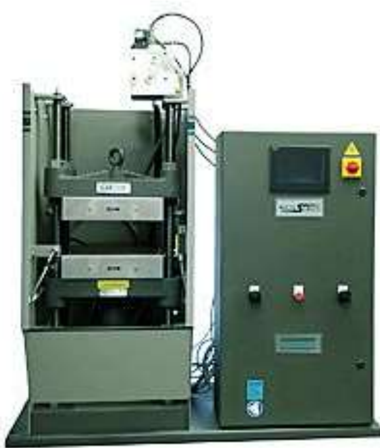
Fig 2.8. Hot Press/Compression Molding.
