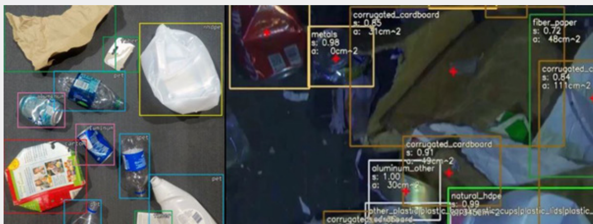
Figure 10: Classification of the material flow of a sorting robot [41,51].
