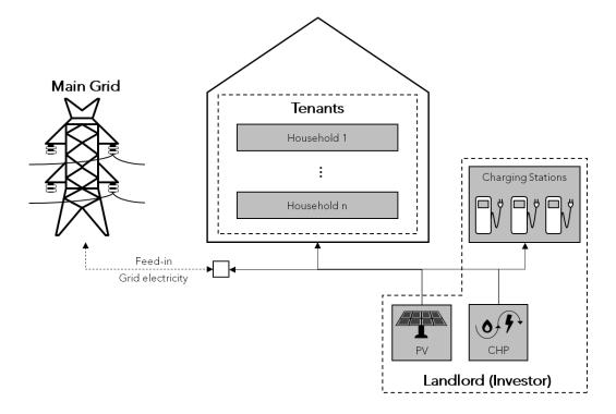
Figure 3: Conceptual Design of a Tenant Electricity Model. Source: (Research Paper 4)
