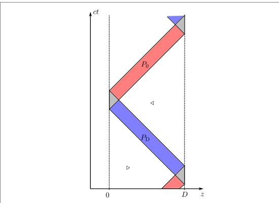
Figure 2. Spacetime is split into zones by the light cones of the reflection events of a pulse oscillating between two mirrors.
