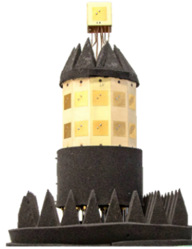
Figure 5.4 Stacked polarimetric uniform circular patch array with 58 ports. We have used only the ports corresponding to the two stacked circular arrays with 12 elements per ring. ■
