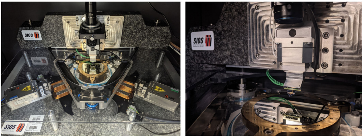
Figure 2: Image of the nanopositioning machine and a mounted tip-based measuring system (left) and detail view of the tip-based measuring system (right) [2].
