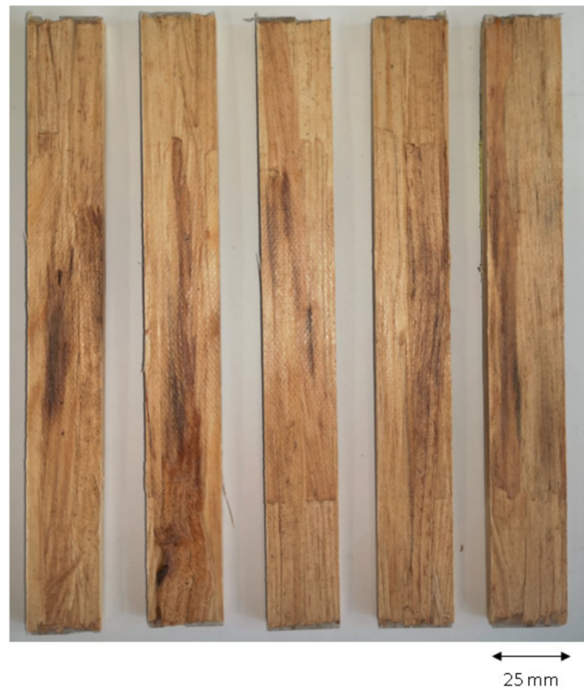
Figure 12. Manufactured WPC specimens for tensile testing.
