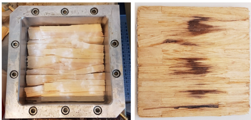
Figure 11. Manual production of WPC specimens consisting of OSB strands and thermoplastic powder.
