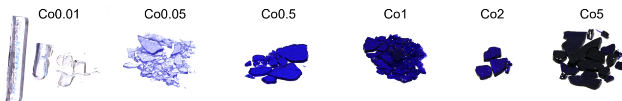
Fig. 5.3: Colour of 45\text{P}_2\text{O}_5-(30-x)\text{CaO}-25\text{Na}_2\text{O}-x\text{CoO} glasses, with 0.01 \leq x \leq 5 mol%.
