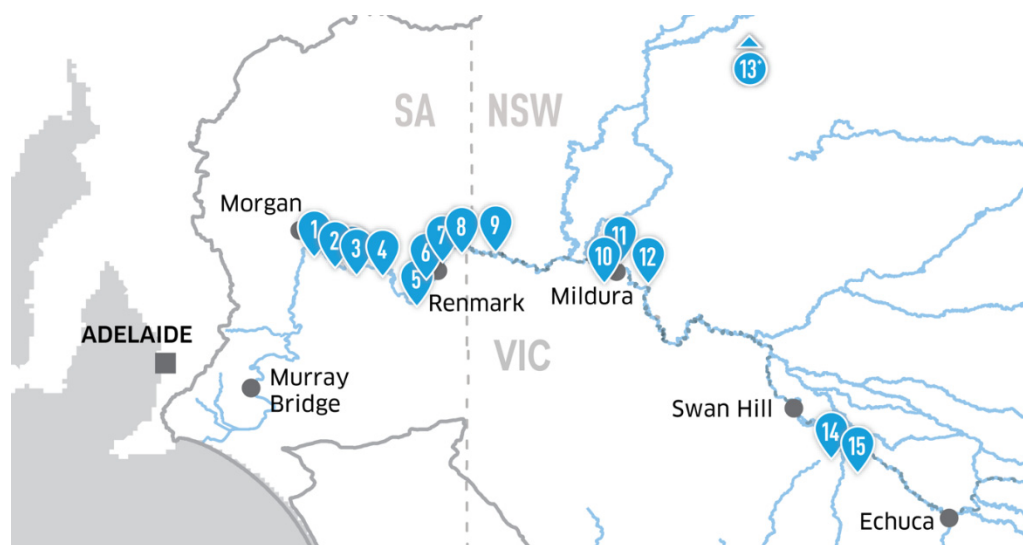
Figure 6. Map of the salt interception schemes in the lower River Murray and Darling River: 1. Waikerie 2A; 2. Waikerie (Lock 2); 3. Waikerie; 4. Woolpunda; 5. Loxton; 6. Bookpurnong; 7. Pike; 8. Murtho; 9. Rufus River; 10. Mildura-Merbein; 11. Buronga; 12. Mallee Cliffs; 13. Upper Darling; 14. Barr Creek; 15. Pyramid Creek. (Source: MDBA).
