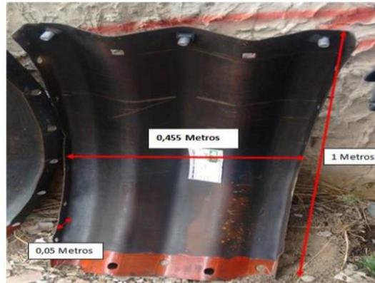
**FIGURA 4.** Dimensiones De Tunnel Liner.
