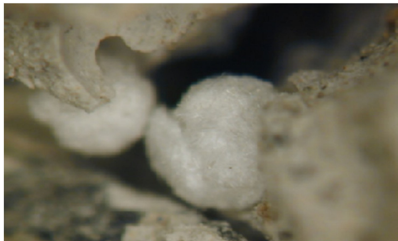
Figure 3. Acicular and white appearance of compounds observed by optical microscopy.
