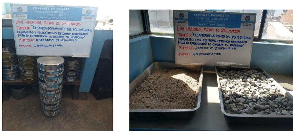
FIGURA 6: GRANULOMETRÍA DEL AGREGADO FINO - ASTM C33-16
