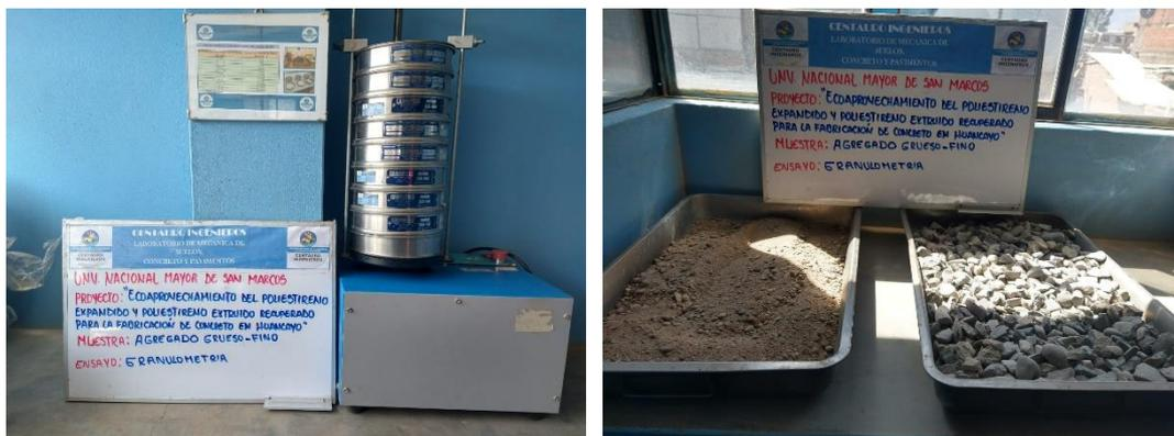
FIGURA 7: GRANULOMETRÍA DEL AGREGADO GRUESO -- ASTM C33-16
