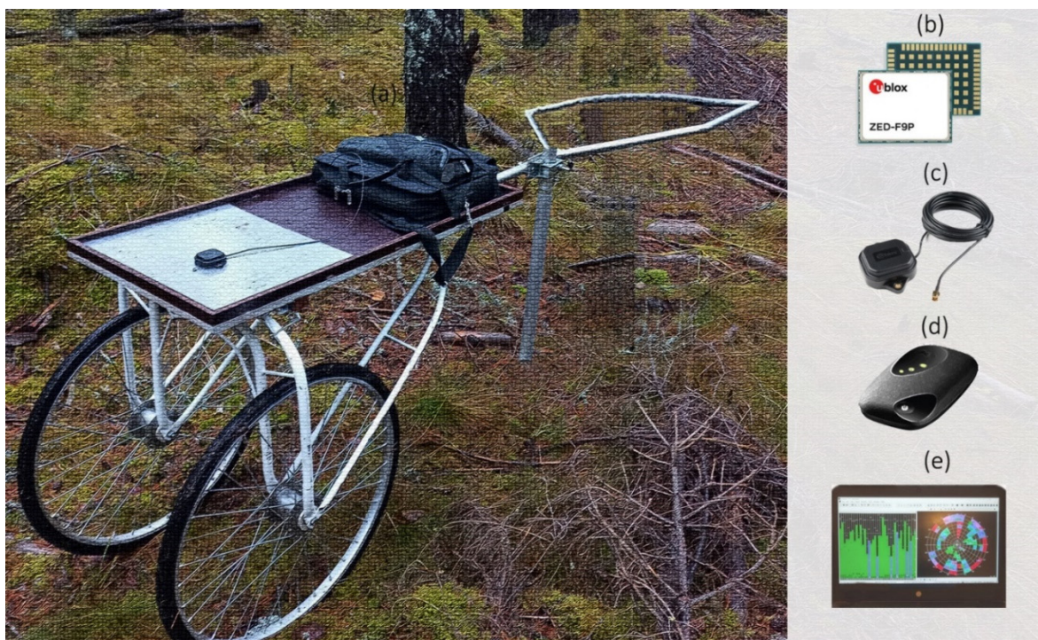
Figure 2. Compartments for field experiment: (a) research sulky, (b) u-blox ZED-F9P, (c) Multi band GNSS antenna ANN-MB-00 (SMA), (d) modem, and (e) computer system.
