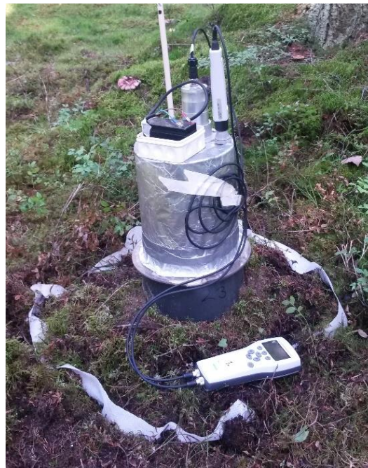
Figure 2. Soil surface respiration chamber darkened with aluminum foil and containing the CARBOCAP® GMP343 CO 2 probe and a data logger on the ground in front. The measurement point is one of the trenched measurement points. Photo: Maiju Kosunen.
