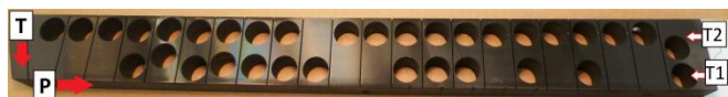
Figure 2: Tile HM58TM200hTE4 after drilling of samples. T and P show the toroidal and poloidal directions of the magnetic field. T1 and T2 represent the samples in the toroidal direction.
