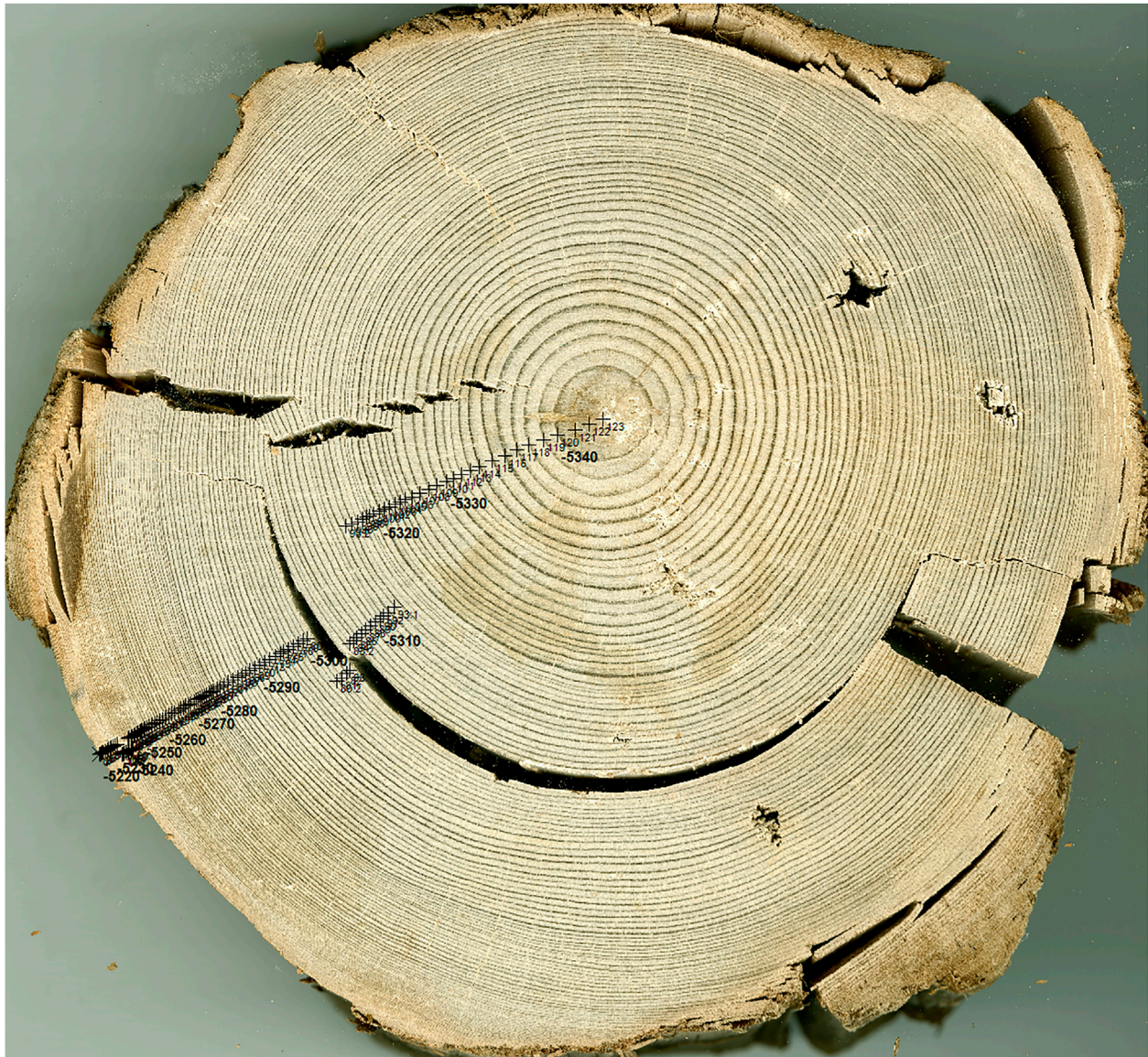
FIGURE 2 | Scanned cross-section of a typical subfossil pinewood sample with tree rings measured in Coorecorder software (Rydval et al., 2014; Maxwell and Larsson, 2021). Measurements of this sample were carried out in three longer and one short separate segment, minding the gap formed during the shrinkage, perpendicularly to ring boundaries. Image by Hannu Herva (22 April 2013).
