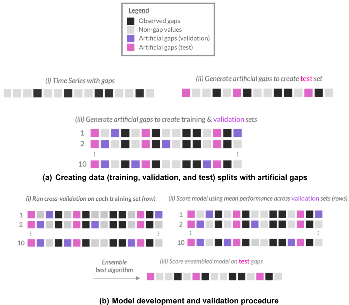
Figure 2. Artificial gap generation and evaluation procedure. (a) Artificial gaps are introduced to create the test set, which is set aside, followed by several alternative validation sets. (b) One model is trained on each validation set, including a 5-fold cross validation step to tune hyperparameters. The validation set performance can be compared across the different algorithms. Then, for select algorithms (best on validation set), the 10-model ensemble is run on the test set to fill in gaps and mean predictions are used to obtain a final score while prediction variance is used to parameterized uncertainty distributions. With this procedure, no model tuning or predictor selection is performed on the test set.
