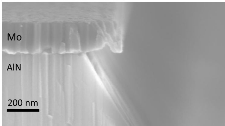
Figure 25. AlN with a Mo mask which was etched and annealed at 700 °C resulting in damage to the edge and increased lateral etching.
