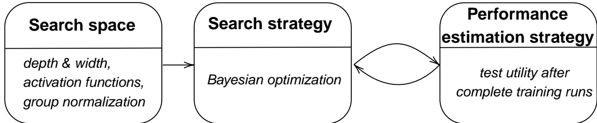
Figure 3.4: Abstract illustration of the neural network search conducted in this thesis. The figure is heavily inspired by the illustration from Elsken et al. [EMH19, p.2].
