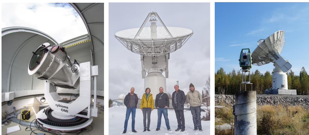
Figure 3. (Left) New SLR telescope, (middle) VLBI radio telescope, (right) local tie and telescope deformations measurement.
