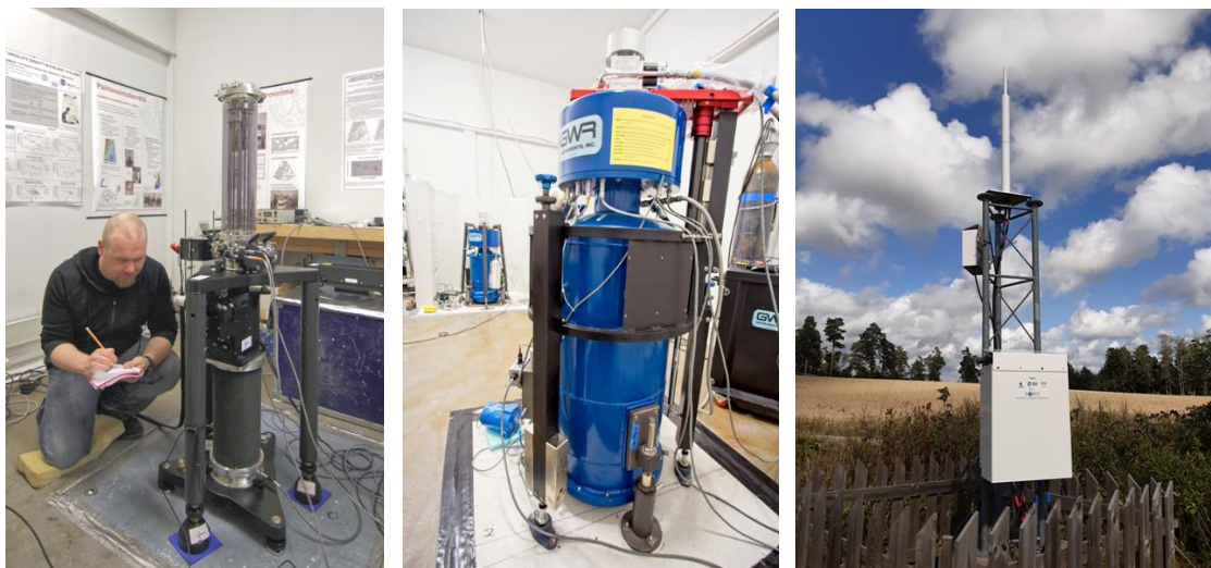
Figure 4. (Left) FG5X-221 absolute gravimeter, (middle) two superconducting gravimeters, and (right) DORIS beacon.
