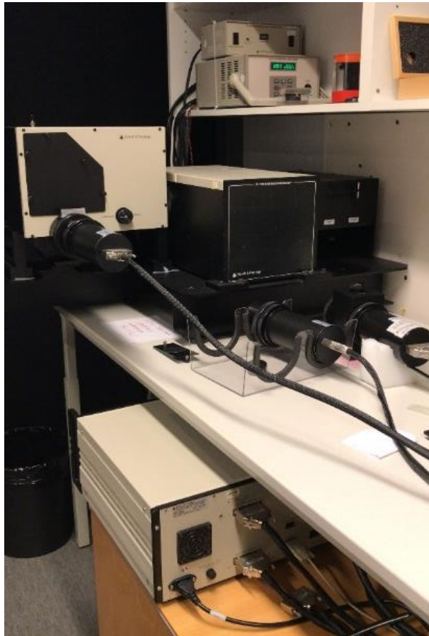
Figure 12. OL-750 automated spectro-radiometric measurement system by Gooch & Housego at the Department of Physics, University of Helsinki
