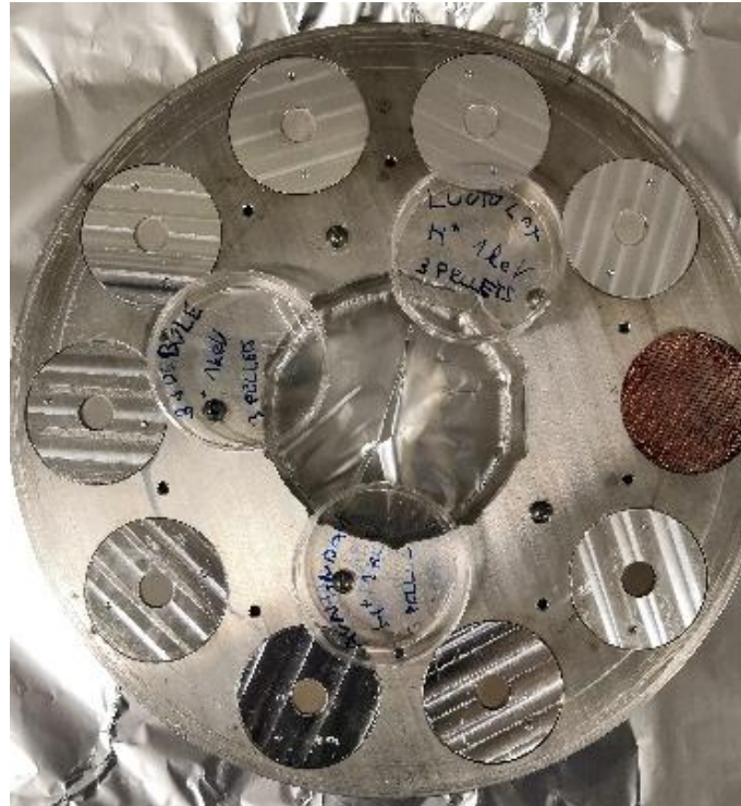
Figure 11: Sample mounted on the sample holder for ion irradiation experiment
