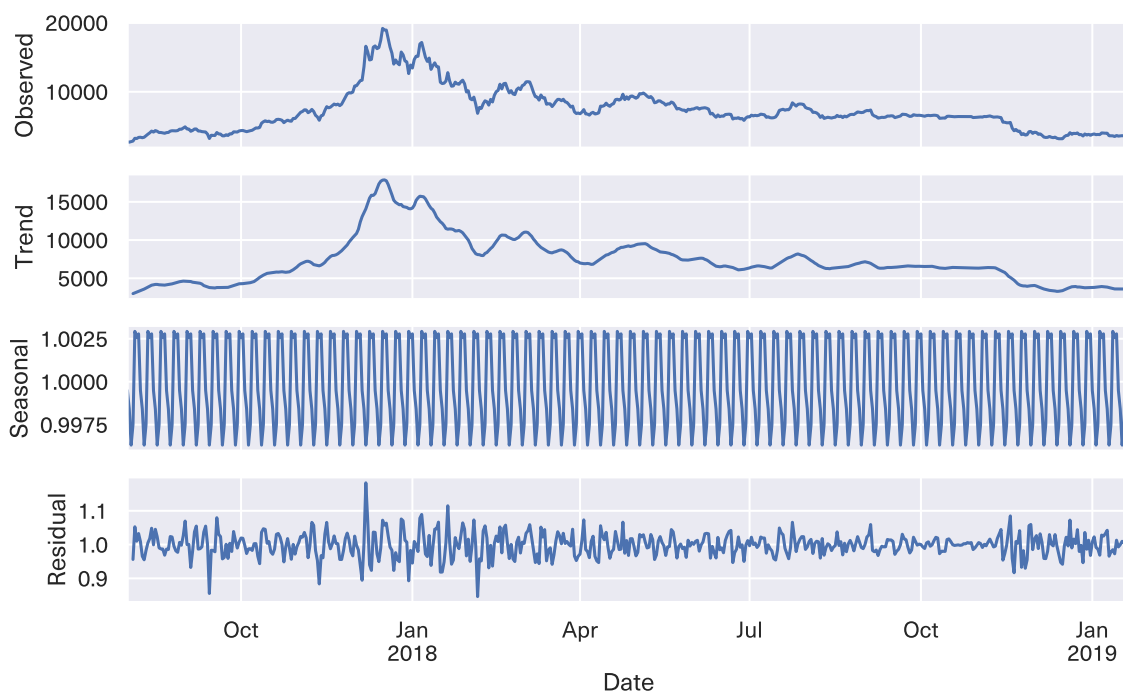
Figure 3.1: Multiplicative time series decomposition of the bitcoin closing price data. The insignificant variation in the Seasonal component indicates that there is no strong seasonal influence on the price of bitcoin.
