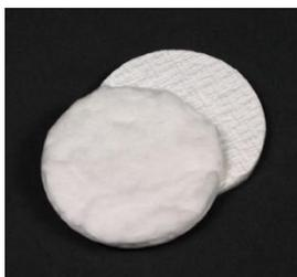
Figure 11: SPE extraction disks usable for extraction of liquid matrices in SFE [74].
