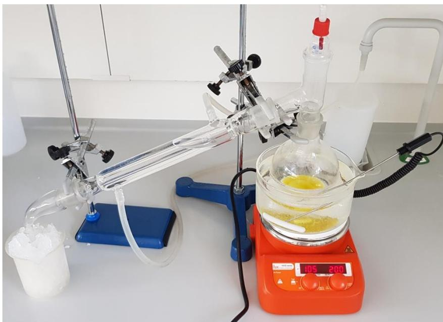
Figure 25: Experimental setup for hydrodistillation of olive oil sample.
