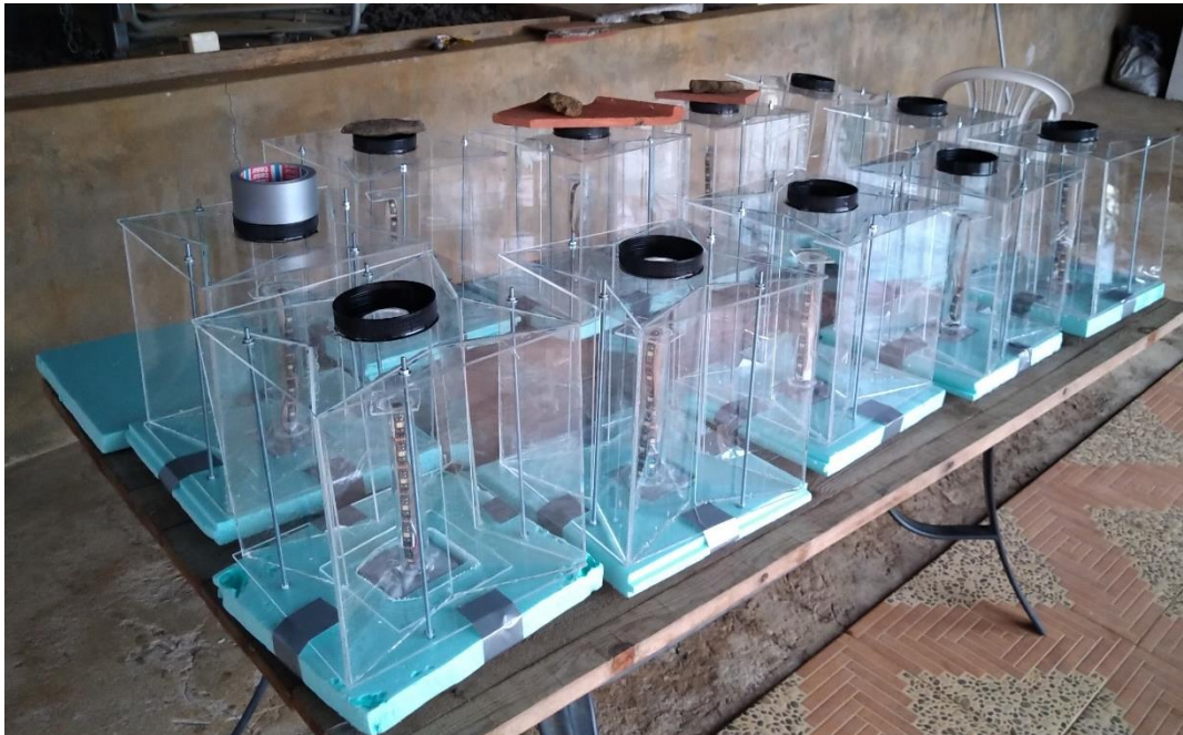
Figure C.1.2 – Light traps in assembly (upside down) with collection jar not attached while being built in São Tomé
