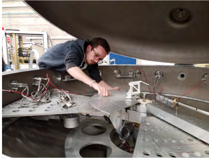
Figure 4.2: Inside view of CT-2000 Chamber. It is possible to see the two rotating arms, some of the flanges with cables and the beam line. On the platform on top of the rotating plate there are two detectors' holding frames.
