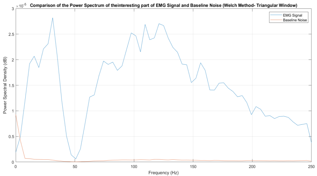
Figure B.8: Pwelch plot of the baseline noise (red line) and the interesting part of the signal (blue line) for volunteer number 29.
