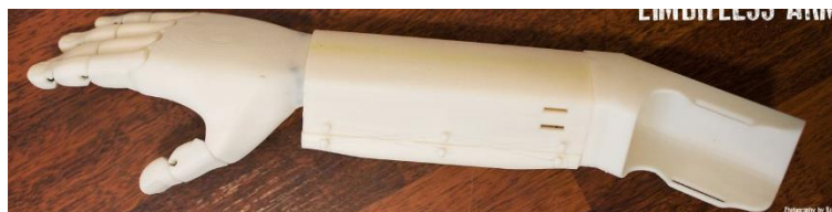
Figure 2.14: Limbitless Arm (extracted from [14])
