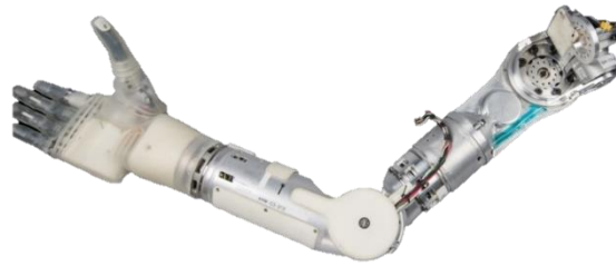
Figure 2.18: DEKA arm (extracted from [72]).
