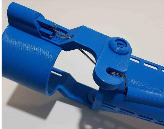
Figure D.4: Tension Mechanism of the fingers (its linked on the forearm and cuff).
