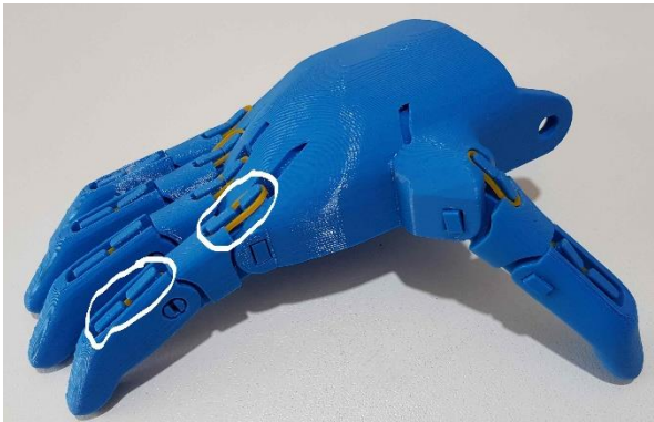
Figure D.3: Elastic Tension Mechanism of the fingers.
