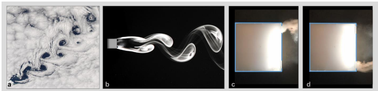
Figure 4.1 – Vortex shedding at different flow scales: (a) – vortex shedding at the cloud level as wind passes through a remote island [112]; (b) – vortex shedding at the wake region of a spanned cylinder [113]; (c) and (d) – smoke visualization of the oscillatory pumping ventilation mechanism (from this study).
