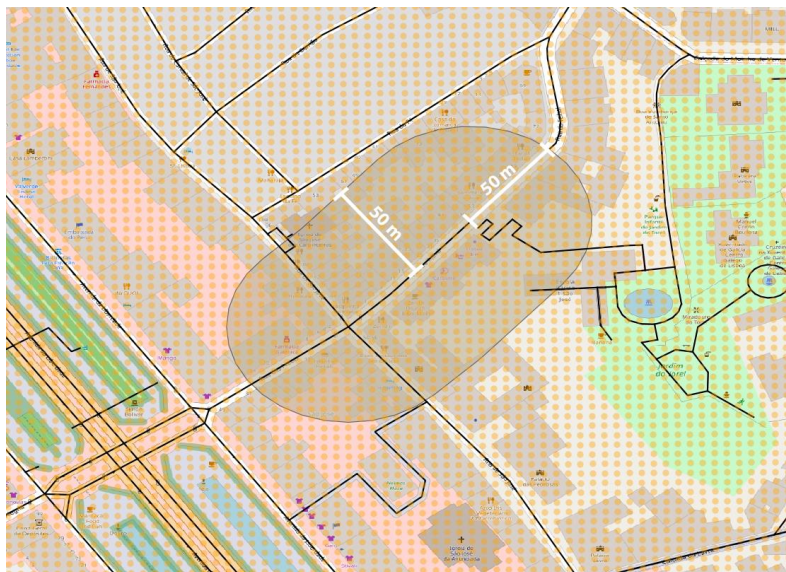
Figure 32 – Example of a buffer of air quality around an edge in QGIS.
