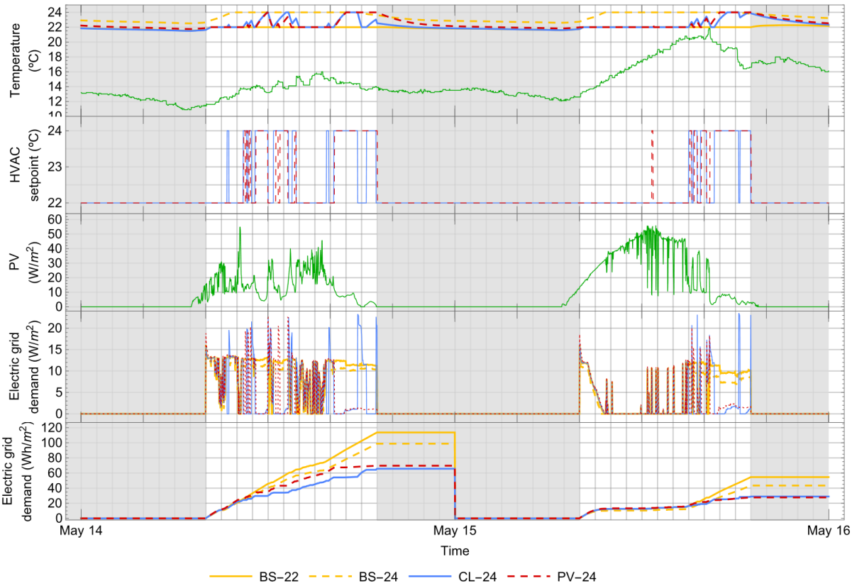
Figure 4.7 Results of the four demand flexibility scenarios for the 14 th and 15 th of May: Air temperature in the ground floor of South open space (1 st row); fan coil cooling setpoint (2 nd row); BIPV production by building floor area (3 rd row); Electric grid demand (4 th row); and accumulated electric grid demand (5 th row). Gray areas corresponds to unoccupied periods.
