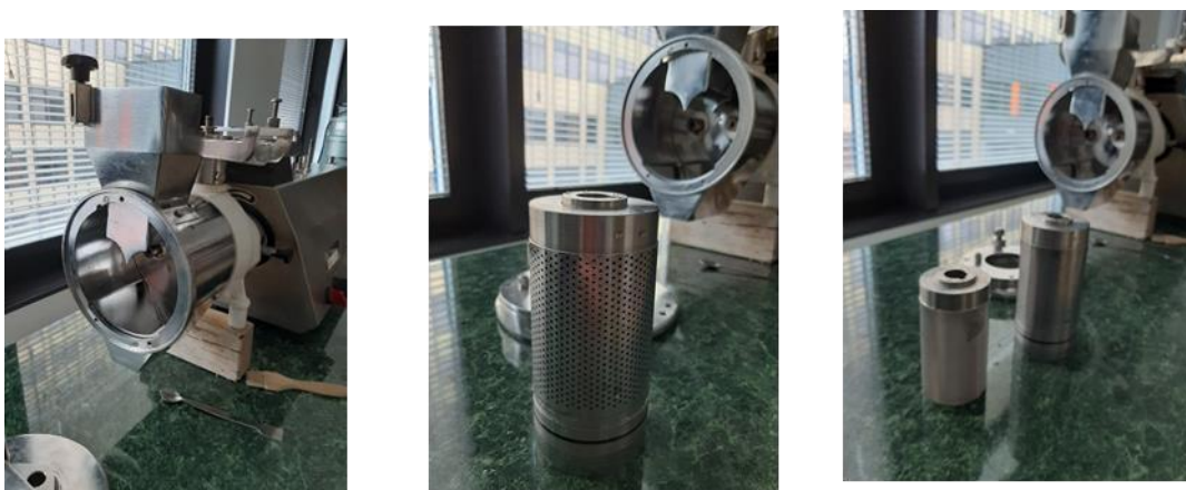
Figure 10 Roll extruder Alexanderwerk Gun with two counter-rotating rollers. Chamber (left), Rollers (Center and right)
