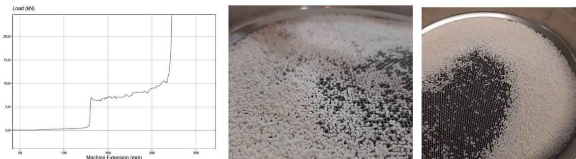
Figure 13 Images related to the production of acceptable quality pellets - curve 'force/displacement' (left), extrudates produced (center) and pellets collected after spheronisation (right), for formulation 12.
