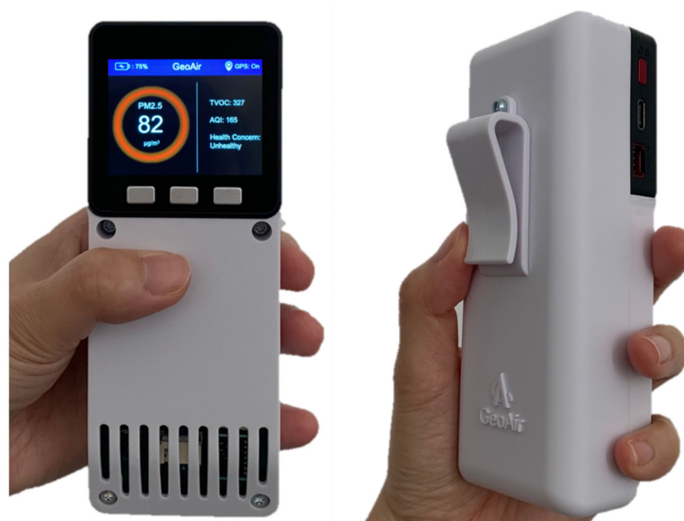
Figure 2. GeoAir2: A portable, GPS-enabled, low-cost air pollution monitor.
