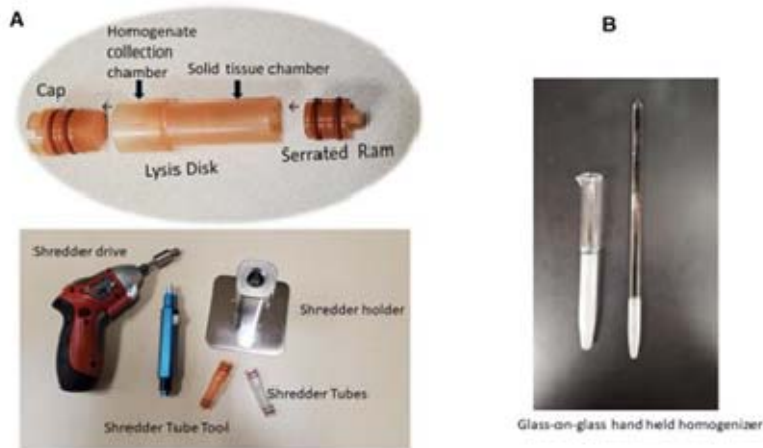
FIGURE-1: Tissue shredder chamber (tube) for use with the shredder.
