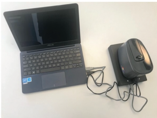
FIGURE 1 Veggie Meter ® instrument and laptop interface.
