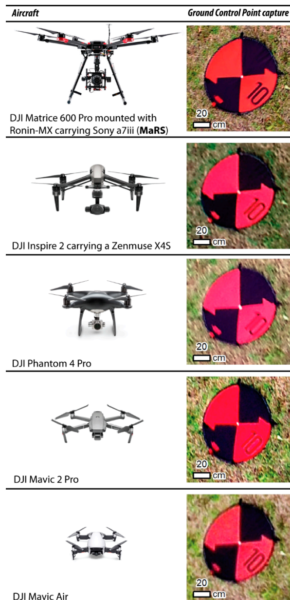
Figure 2. The five aircraft used in this study along with an example of each camera's ability to capture a Ground Control Point (GCP). Aircraft image source: https://www.dji.com/ (accessed on 10 October 2020).
