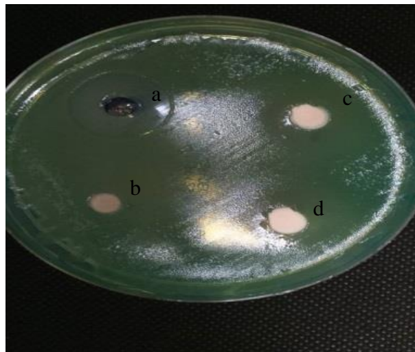
Figure 4.18 Inhibition zone for a) Chlorhexidine b) pure PMMA c) PMMA/15% \beta -TCP/2.5% ZnO and d) PMMA/15% \beta -TCP/5% ZnO against P. aeruginosa .
