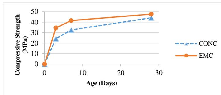
**Figure 4.** Compressive strength development for EM and control concretes.
