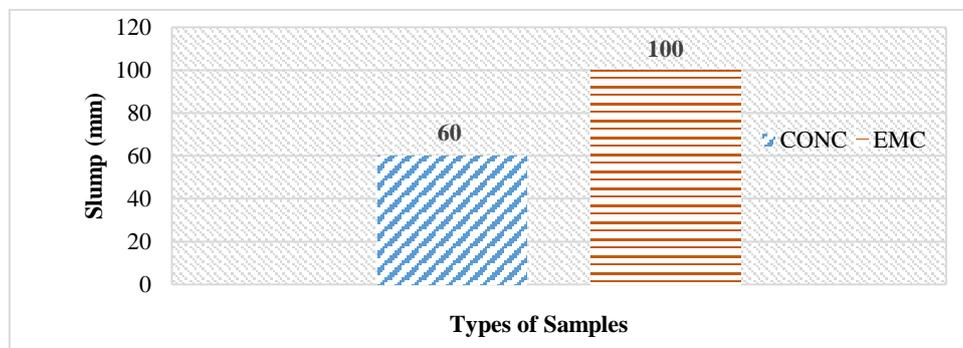
**Figure 2.** Workability of EM and control concretes.
