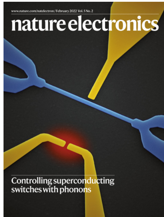
Figure A.1. Cover Nature Electronics, Volume 5 Issue 2, February 2022. False colored SEM micrograph of a TiN nanowire (blue) on a Si substrate, together with TiN gates (yellow). Image: Markus F. Ritter, cover design: Allen Beattie. Copyright 2022 Springer Nature.
