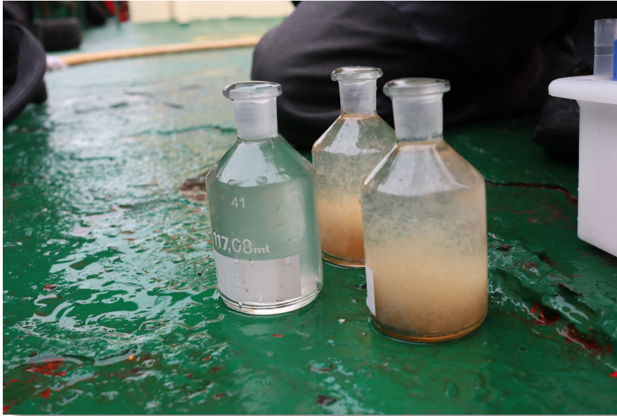
Fig. 7.2: Glass bottles prepared for Winkler titration, photo: A. Krönert
