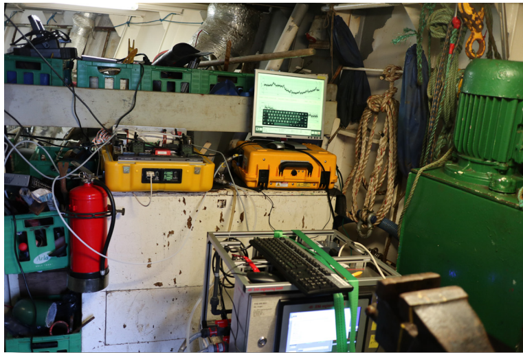
Fig. 7.3: Setup of the FerryBox and LosGatos Analyser in the ship's bow; photo: A. Krönert
