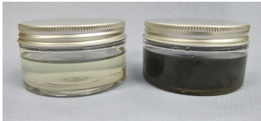
Figure 4. Gear oil before (left) and after (right) the oil was exposed to harmful EDM discharges in a modified bearing test rig.
