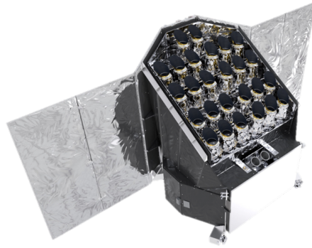
Figure 1. Artist impression of the PLATO Spacecraft with the 26 cameras on the optical bench. The Electronic Units are hidden behind the radiator visible in front below the cameras. Credits: OHB System AG
