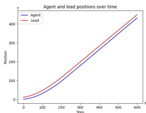
Figure 1. Positions of agent (blue color) and the leading vehicle (red color) over each step from the simulation in meters.
