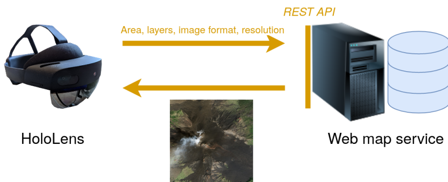
Figure 4.3.: GIS application running on HoloLens, requesting landscape data of a specified area.
