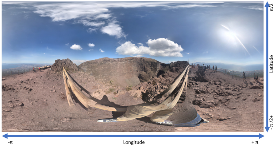
Figure 4.19.: Equirectangular panorama describing a spherical environment. Pixels on the same row are equal in their latitude. Pixel in the same column are equal in their longitude.
