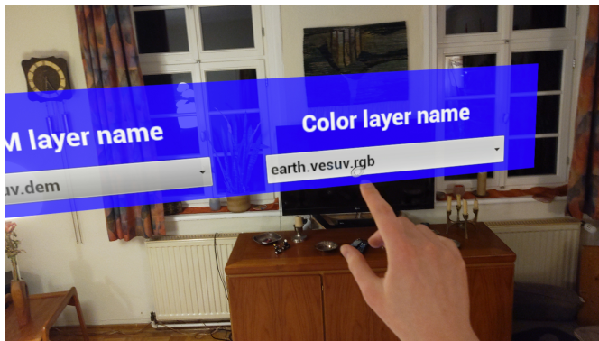
Figure 5.13.: User is selecting the DEM layer (left) and the color layers (right) to be loaded from two drop-down menus.
