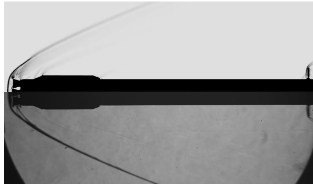
Figure 11: Schlieren photograph comparison for Mach 3.6 baseline case
