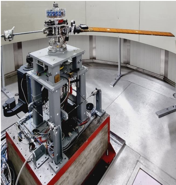
Figure 5: STAR blade in the whirl tower.
