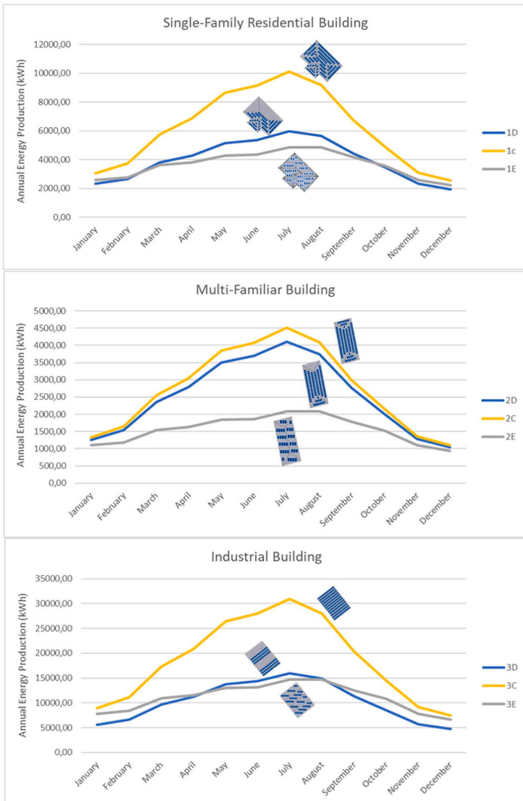
Fig. 11. Evolution of the annual energy production for different building uses as a function of the different solar panel installation configurations.
