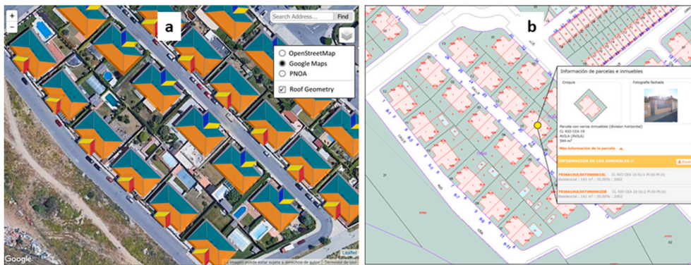
Fig. 2. (a) Layer with geometric information of existing roofs superimposed on the orthoimage from Google Maps and (b) graphic viewer of the cadastral cartographic database linked to Ener3DMap-SolarWeb Roofs.
