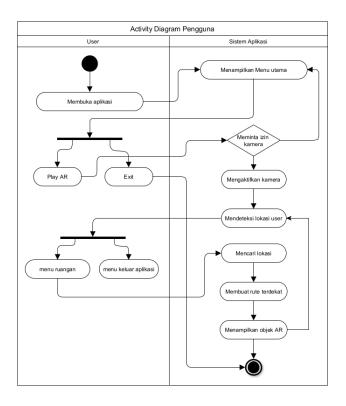
FIGURE 1. User Activity Diagram for AR Applications
